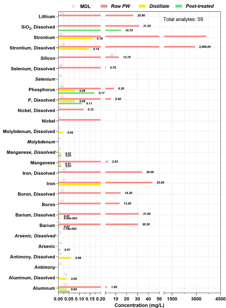
Fig. 4. Targeted characterization of total and dissolved metals in raw PW, MVR distillate, and post-treated water by GAC and zeolite; Out of 59 analyzed metals, 32 were not detected in all water samples.
