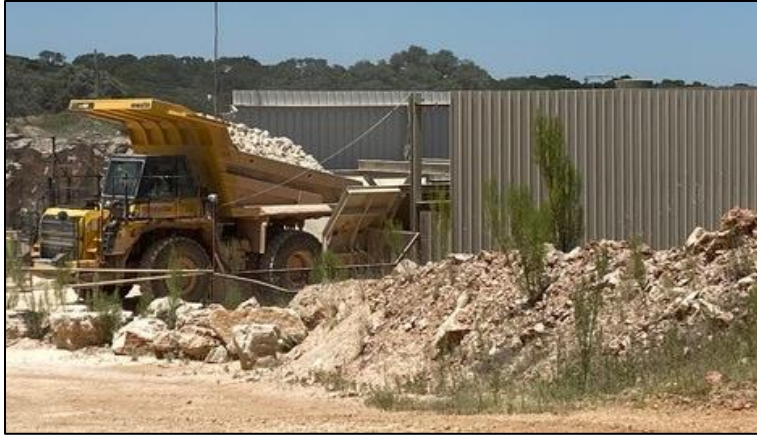
Figure 23. Enclosed Rock Crusher to Control Dust. Source: Jill Shackelford
