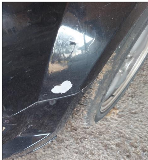
Figure 14. Damage to Vehicle Paint from Rocks Falling Off Aggregate Truck. Source: CREAM
