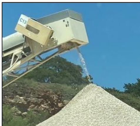
Figure 22. Water Mister at Conveyer Belt Drop Point to Control Dust. Source: Jill Shackelford
