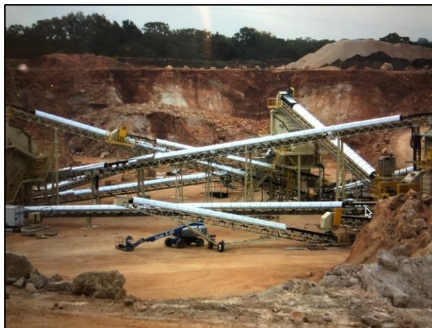
Figure 21. Covered Conveyor Belts to Control Dust. Source: Jill Shackelford
