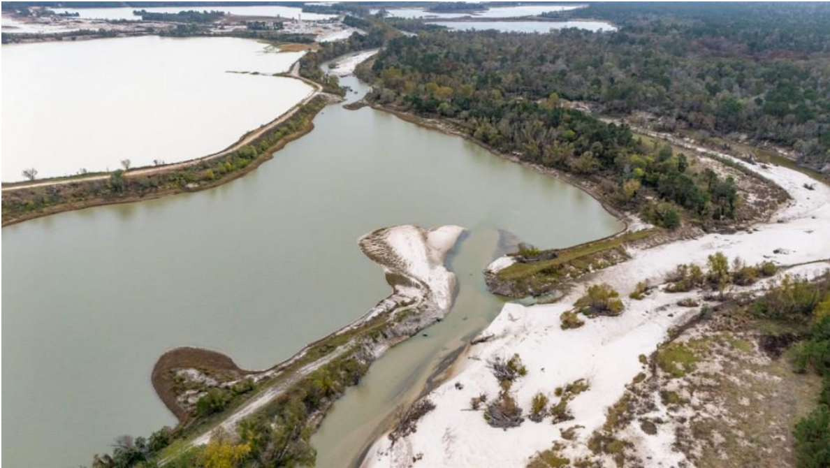
Another West Fork pit capture at the Hallett Mine after floodwaters receded. Notice how natural channel of the river has been virtually cut off.
