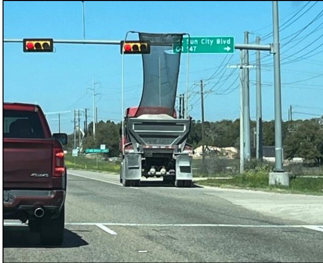
Figure 12. Example of Aggregate Truck with Tarp in the Wrong Position. Source: CREAM
