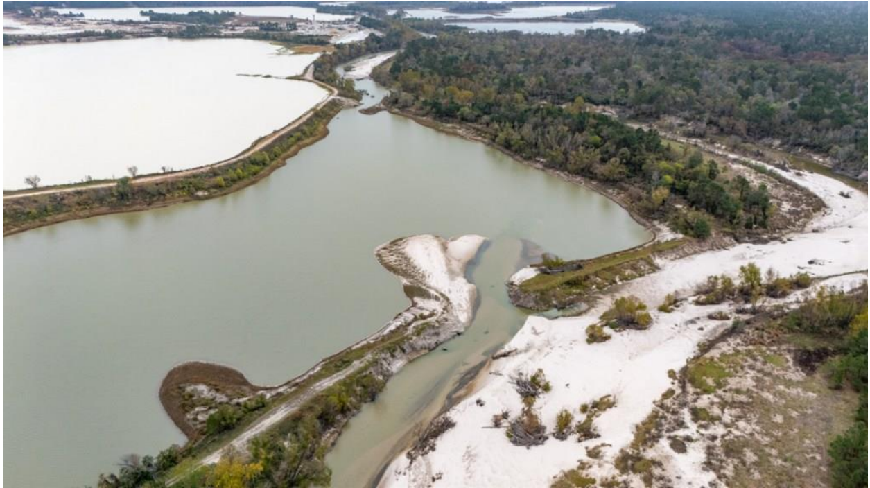
Another West Fork pit capture at the Hallett Mine after floodwaters receded. Notice how natural channel of the river has been virtually cut off.
