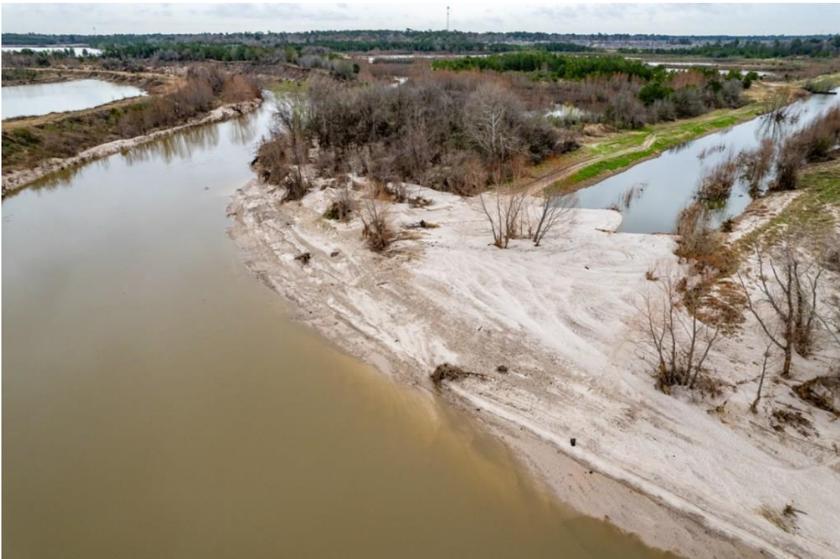
Same ditch blocked by sand increases flood risk for homes (visible in top right).
