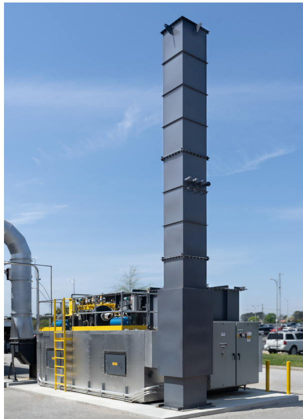
The Oxi.X RM RTO offers the economic advantages of regenerative thermal oxidation exclusively for low-flow process applications.
